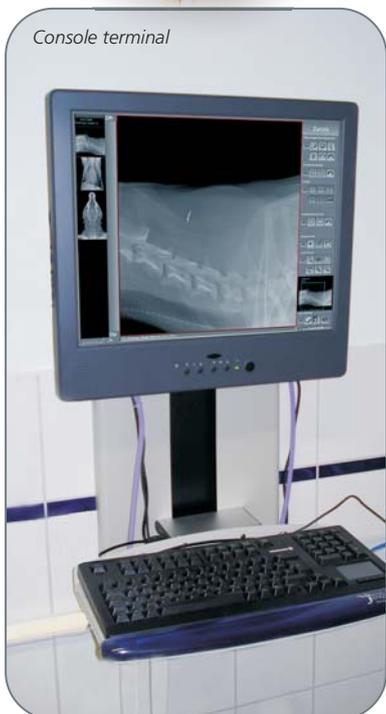
The upgrade made it possible to integrate the existing high-value X-ray unit of the firm of Sedecal into the new direct-digital system. Modifications were not necessary since the raster drawer was simply replaced by the built-in detector."
